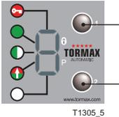
Browse through the fault display using selector key 1 upwards (to display several faults).
