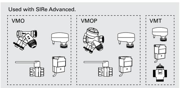
Valve kit VOS(P), VOT, VMO(P) or VMT is used to control the water flow. For more information see the "Controls" section.
