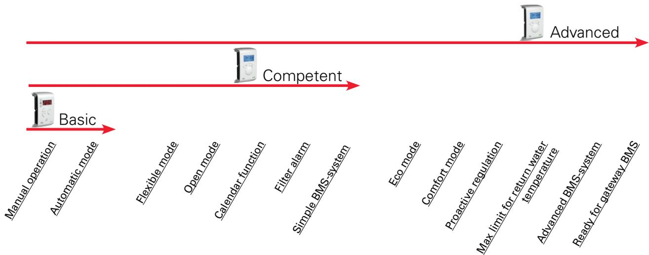
This air curtain is supplied with an integrated PC board SIRE. There are three different levels with different functionality to choose from, Basic, Competent or Advanced. Read more about the SIRE control system in the "Controls" section.
