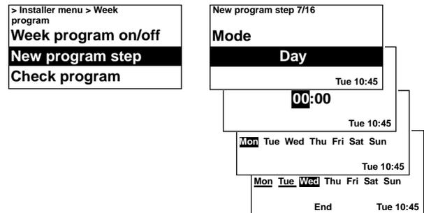
A new program step does not replace a set time for Day for example, but you can instead select to change a program step.
