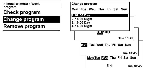
The program steps that should not apply are removed in Remove program. One or all program steps can be removed in the menu. To return to the factory set basic program, select Reset all.
