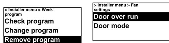
Week program is activated by selecting On, under Week program on/off. In On-mode, a sun, moon or Off in the Status window appears to indicate day, night respectively Off-function.
